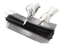
At a notch, cut a length equivalent to the perimeter required plus an overlap of 5 to 6 cm (2") for joining 2
