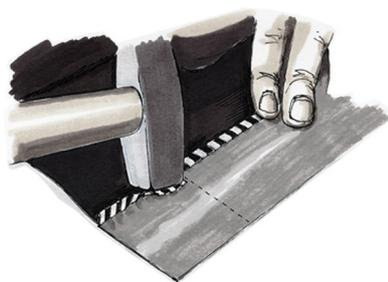
Bend down the seam whilst ensuring that the cloth remains fastened
