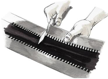
At a notch, cut a length equivalent to the perimeter required plus an overlap of 5 to 6 cm (2") for joining
