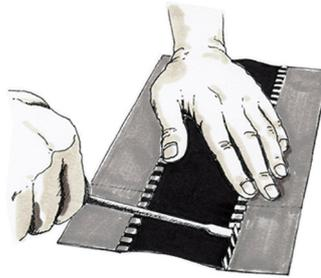
Lift the seam outwards at right angle
