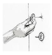
If necessary, cover the pin with protective cap.
