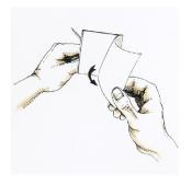
Remove the protective release paper taking care not to touch the adhesive
