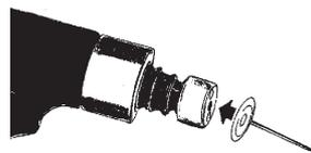
Place the weldfastener CDF on the magnetic head of the gun. Adjust the voltage according to the type and thickness of the sheet metal.
