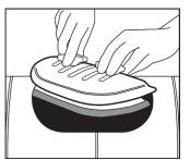
3. Install door by unscrewing the 4. Turn straight and pull out slighlty hand knobs until thread is level to align. Then tighten knobs. with top of bolt. Using both hands place the door in the hole at an angle.
