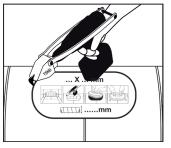
2. Using Turbo Shears or similar cut around template taking care not to exceed the size of the template (the door will function correctly when cut to template size +0 mm -3 mm).
